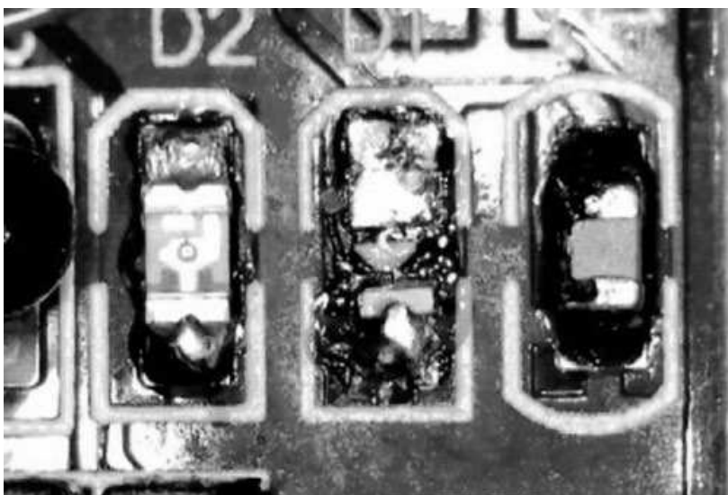
Figure 6-5. LED D_1 removed
