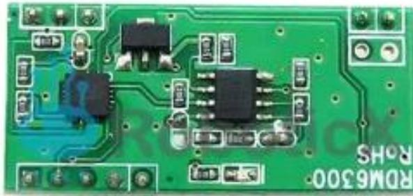
RDM6300 125KHz card reader mini-module is designed for reading code from 125KHz card compatible read-only tags and read/write card . It can be applied in office/home security, personal identification, access control, anti-forgery, interactive toy and production control systems etc.
