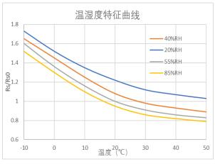
Fig4.Typical temperature/humidity characteristics
